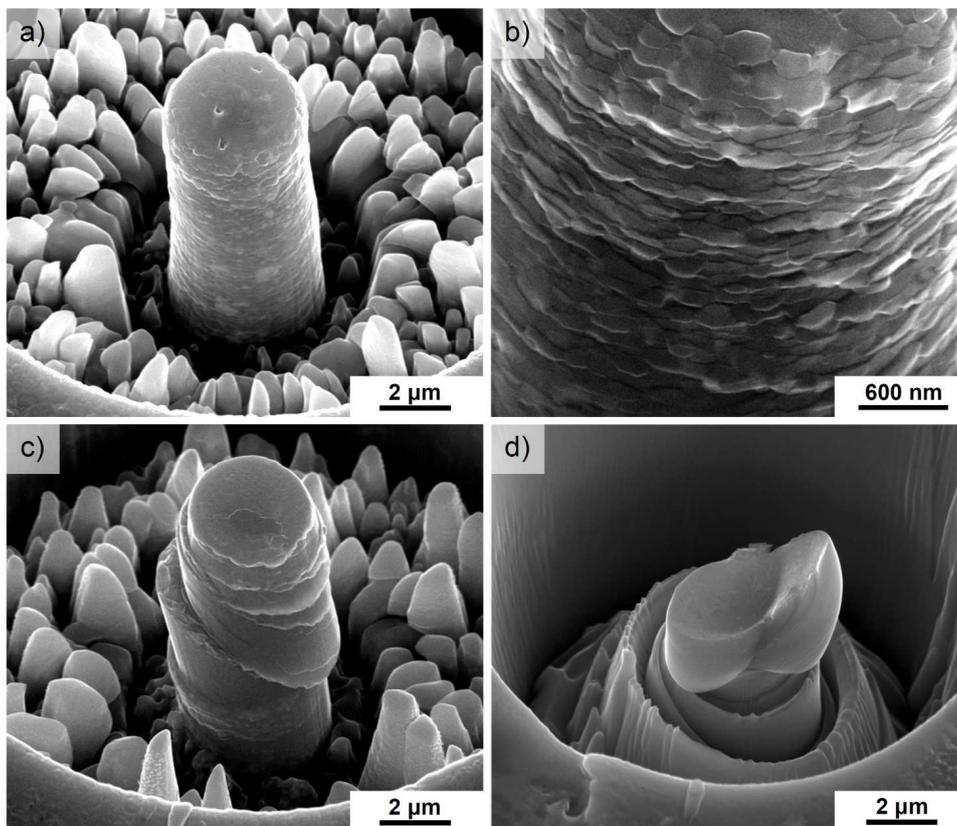
*Figure 5: Surface morphologies of compressed micro-pillars for HPT-processed Al-30Zn in low and high magnifications shown in a) and b), respectively, c) HPT-processed Al-10Zn [15] and d) annealed, coarse-grained Al-30Zn [14] samples.*
