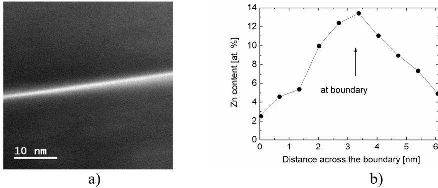
Figure 2: Zn-rich layer at an Al/Al grain boundary in the HPT-processed Al-30Zn alloy, demonstrated by a) TEM and b) EDS results [14].
